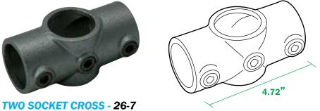
This component is used where two recycled PVC Counter Weights need to be joined together to form a counter weight end detail. Material: Malleable cast iron to ASTM A47-77-32510 and galvanised to ASTM 153.. Net weight: 1lb 6oz.
