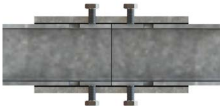
Correct alignment - Top view
