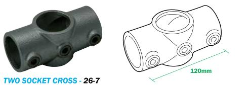
This component is used where two recycled PVC Counter Weights need to be joined together to form a counter weight end detail. Material: Malleable cast iron to BS 1562 and galvanised to BS EN ISO 1461. Net weight: 0.63kg.
