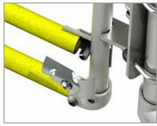
**8.** Mount clamps on lower part of gate; attach mid rail to gate.
