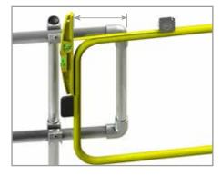
**3.** Measure distance from edge of gate to guardrail upright, and record distance to cut.
