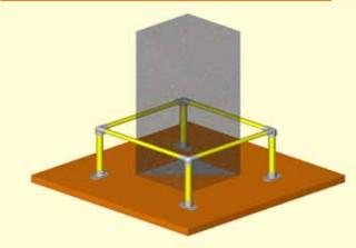
KwikCG1 is a Column Guard manufactured from 48.3mm diameter galvanised steel tube, 800mm square with four uprights and flat fix baseplates.
