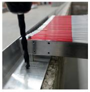
Remove spring loaded bolts if vertical location pin required. Allow enough depth for location pin to fully insert.
